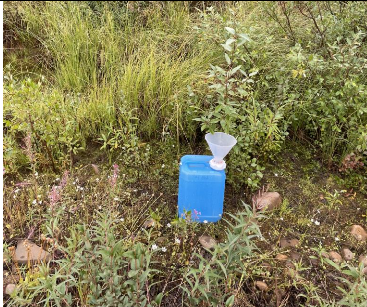
Figure 2. Dust collection trap used to measure how far from the road dust was travelling across the landscape.
