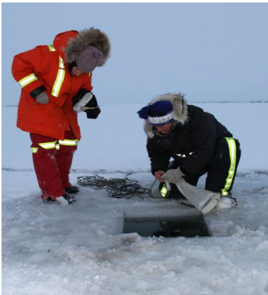
Equipment is lined up at Canadian Helicopter's ready to fly to the field. At the lakes, holes were drilled using a power auger and extended using an ice-saw. Data and samples were obtained through the ice (YSI profiles, water and sediment samples, zooplankton etc) by Shannon M. and Klaus G.. Day light was one limiting factor, but thanks to accurate landings that made lake access easy, pilots provided maximum time on the lake and assured timely returns to
