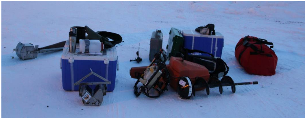
Equipment is lined up at Canadian Helicopter's ready to fly to the field. At the lakes, holes were drilled using a power auger and extended using an ice-saw. Data and samples were obtained through the ice (YSI profiles, water and sediment samples, zooplankton etc) by Shannon M. and Klaus G.. Day light was one limiting factor, but thanks to accurate landings that made lake access easy, pilots provided maximum time on the lake and assured timely returns to
