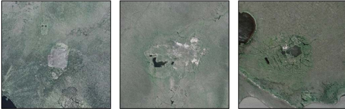
Figure 4. Examples of drilling-mud sumps and lease areas showing varying magnitudes of terrain subsidence caused by ice wedge degradation, Mackenzie Delta region, Canada. (1) Site 1 is in the tall shrub transition zone and shows no evidence of ice wedge subsidence; (2) Site 2 shows minor to moderate subsidence due to ice wedge degradation; and (3) Site 3, located in the dwarf shrub tundra is the most northerly site and has experienced major surface subsidence and ponding due to ice wedge degradation.
