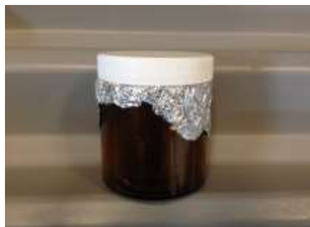
FIGURE 11 – Properly covered iChem jar with polyethylene tape inside.
