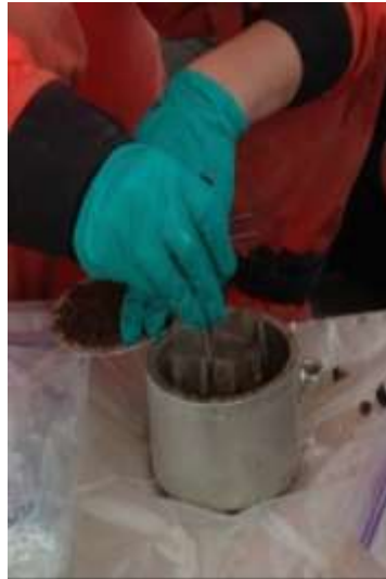
FIGURE 10 – Removing polyethylene tape from PMD
