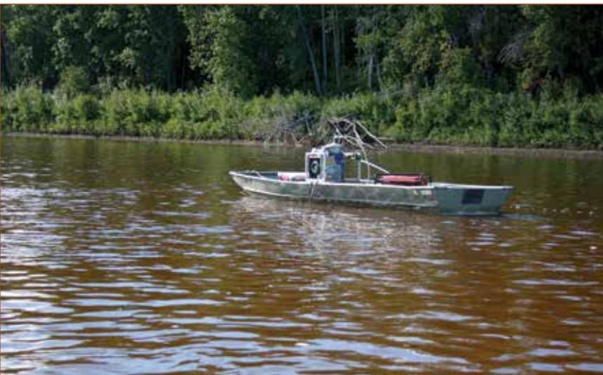
Centrifuge equipment mounted on boat anchored in the river. Centrifuge runs for up to 24 hours and collects the suspended sediment from the river. Both the suspended sediment and water are analyzed for many different substances, including metals and hydrocarbons.
