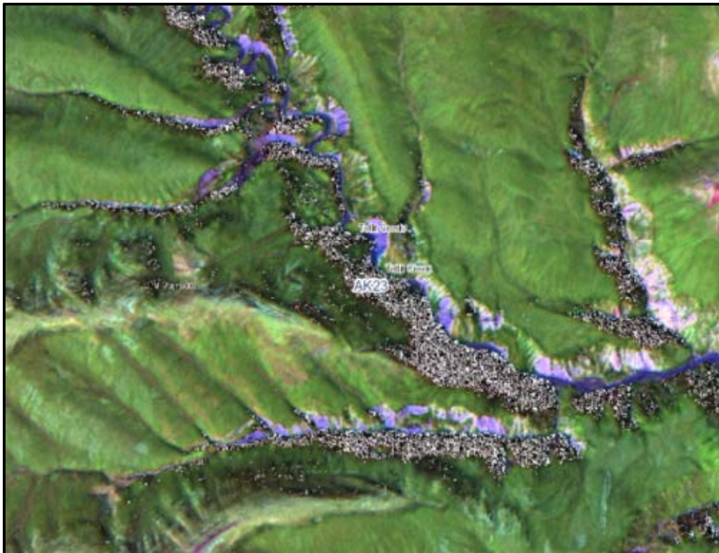
Figure B3. SPOT imagery showing part of Tetlit Creek. The meandering creek has eroded a canyon, creating small cliffs with cusped tops, which could be mistaken for slumps.
