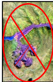
Figure B10. Incorrect measurement of slump scar length. This measurement was taken across the slope.
